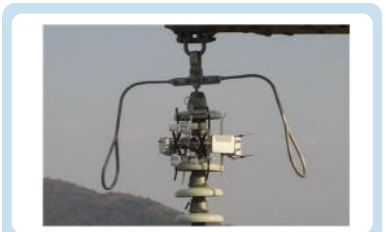
Inspection using live insulator inspecting robot
