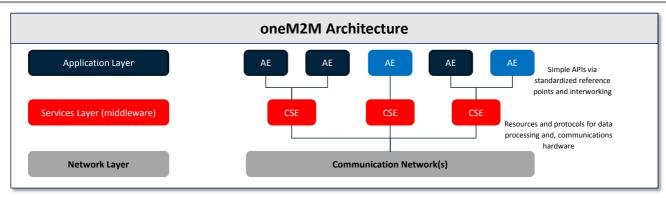
Application Entities (AEs) within individual device and sensor applications provide a standardized interface to manage and interact with applications.
