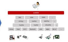
By implementing oneM2M CSL, at the device and the infrastructure side, the developer only uses the globally specified oneM2M APIs to push data from the device into the cloud.
