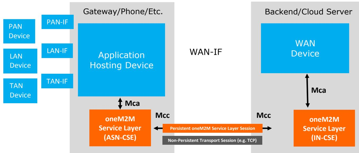
oneM2M Service layer hosted on AHD registers to service layer hosted on WAN Device. This registration persists independently of underlying transport session being setup and torn-down.
